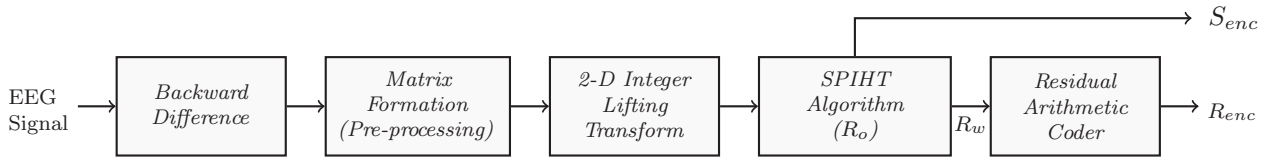
Fig. 8. Two-stage coder for EEG compression: first lossy-stage is SPIHT encoder until an optimal rate ( R_0 ), followed by arithmetic coding for residuals.
