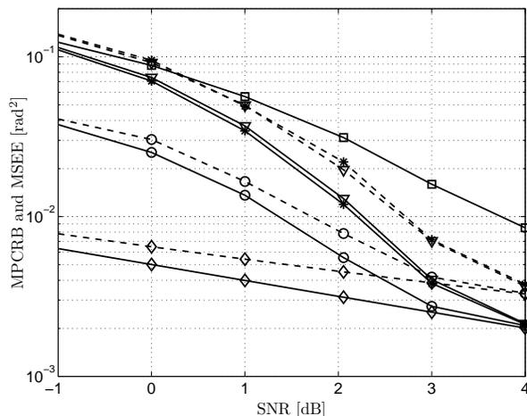
Figure 7: MPCRB and MSEE for  $\sigma_W^2 = 0$  and  $\sigma_W^2 = 10^{-4} \text{ rad}^2$ ; shown are (1) the MPCRBs of [16] (diamonds); (2) the MSEE of the particle based (circles), EM based (stars), and the sum-product steepest descent based (triangles) synchronizers; (3) the MSEE of the M-law (squares), only for  $\sigma_W = 0$ .
