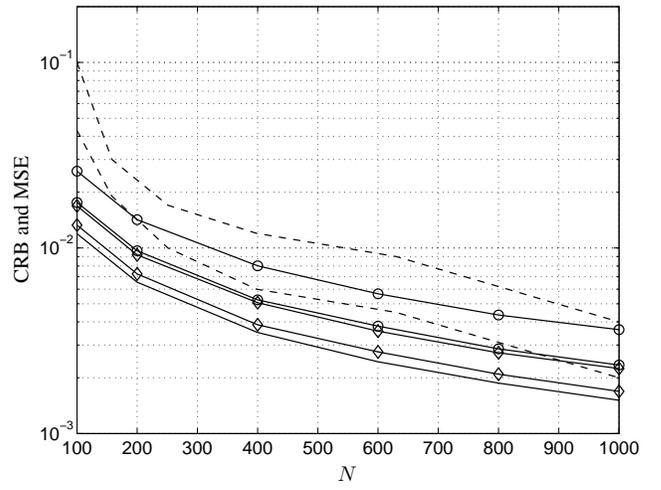
**Fig. 2.** CRB for coefficient estimation. Shown are (1) LPC-algorithm with known  $\sigma_U^2 = 0.1$  and  $\sigma_W^2 = 0$  (solid line); (2) Grid-based algorithms of [10] with unknown  $\sigma_U^2 = 0.1$  and unknown  $\sigma_W^2 = 0.01$ , and 0.001 (dashed); (3) CRB for known/unknown  $\sigma_U^2 = 0.1$  and known/unknown  $\sigma_W^2 = 0.01$  (circles), 0.001 (diamonds).
