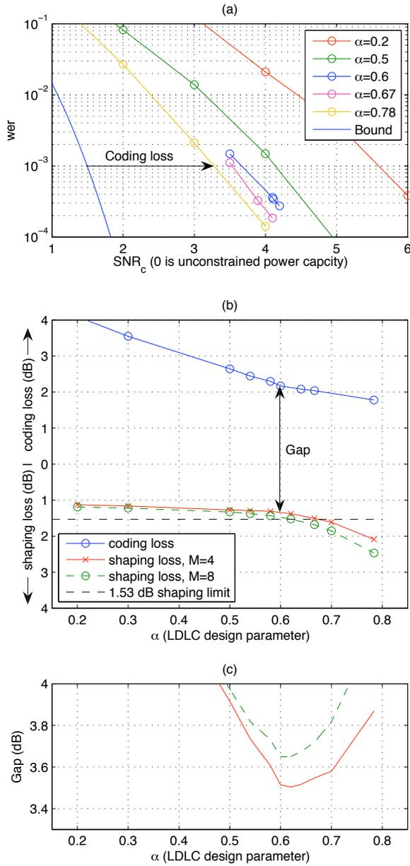
Fig. 2. Design of LDLC lattice codes with  $n = 100$ ,  $d = 3$ . (a) Coding loss for  $\Lambda_c$ , on unconstrained power channel. (b) Coding loss (from (a) at error rate  $10^{-3}$ ) and shaping loss (based on Monte Carlo integration;  $Q = 10$  was used) versus lattice parameter  $\alpha$ . (c) Sum of coding loss and shaping loss, that is, the gap in (b), and a minimum is observed around  $\alpha = 0.6$ .
